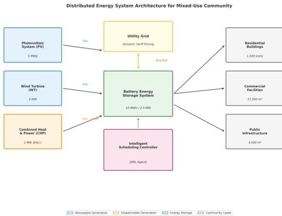
Fig. 2. Architecture of the Distributed Energy System, showing the interplay between generation sources, storage, community loads, and the utility grid.
