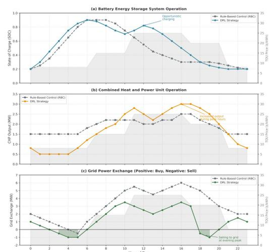
Fig. 5. Comparison of system operation on a typical day under the TOU tariff, contrasting the DRL strategy with the RBC baseline across (a) BESS operation, (b) CHP dispatch, and (c) grid exchange.
