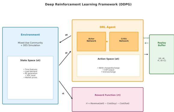
Fig. 4. The Deep Reinforcement Learning framework, illustrating the interaction between the DRL agent (Actor-Critic networks) and the environment.
