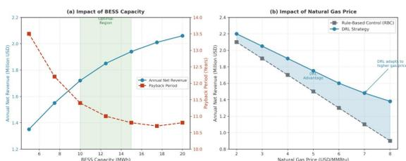
Fig. 7. Sensitivity analysis showing the impact of (a) BESS capacity on annual revenue and PBY, and (b) natural gas price on annual revenue for both strategies.
